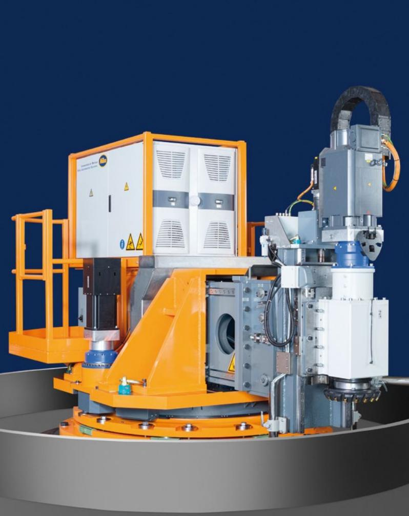
Powerful Mobile CNC Milling Machine for steel towers
