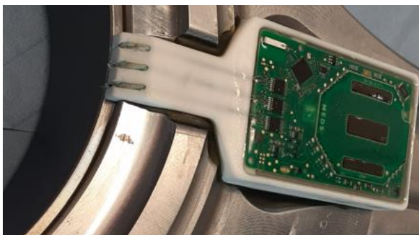
Figure 27. Picture of the Miba telemetric system with 3 thermocouples mounted on a HiPo engine connecting rod
