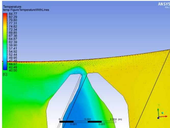
Fig 10 – Hydraulic back flow of fresh oil in an oil supply unit with longitudinal slit according to design E3.
