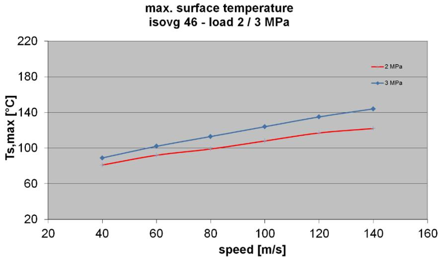
Fig 1 – Example for increase of max. surface temperature of sliding pad related to circumferential speed
