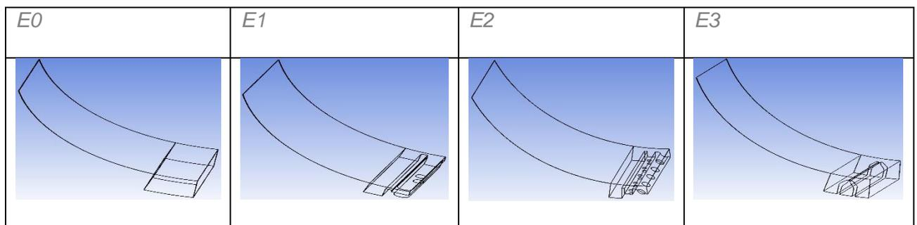
Tab1 – Different units for oil supply: E0: Simple oil supply (flooded lubrication); E1: Supply unit with dam and tank; E2: Supply unit consisting of oil drainage, dams, injections; E3: Supply unit consisting of dam and longitudinal slit.
