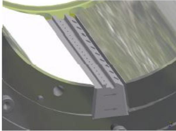
*Fig 5 – Three-dimensional presentation of a tilting-pad bearing; space between pads filled by means of oil drainage, dams and oil injection unit according to design E2.*
