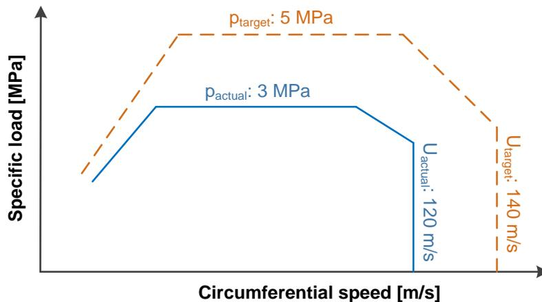
Fig 2 – Combination of specific load and circumferential speed of a tilting pad bearing application – usual limits may be shifted in future applications
