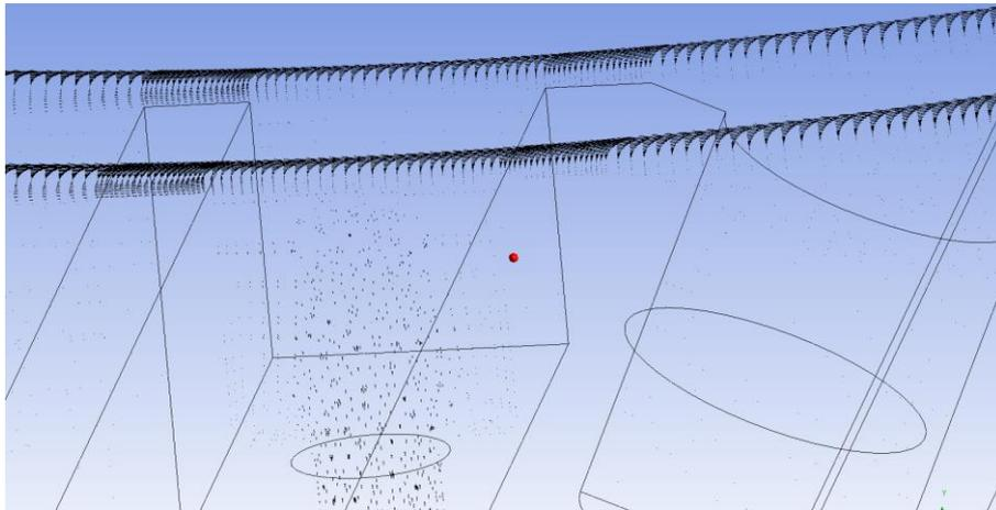
*Fig 8 – Distribution of oil flow in an oil supply unit according to design E2. Separation of flow back of fresh oil by means of the first oil injection.*
