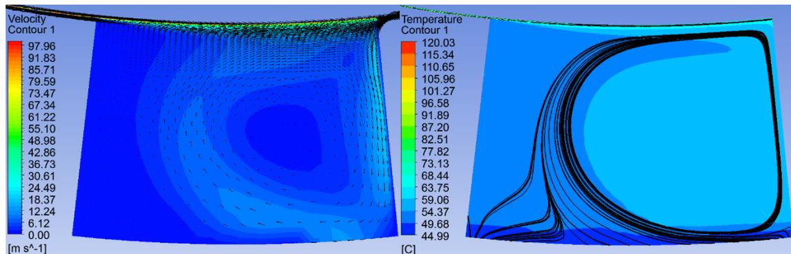
Fig 4 – Distribution of velocity and temperature in an oil supply pocket according to design E0 presented by CFX simulation
