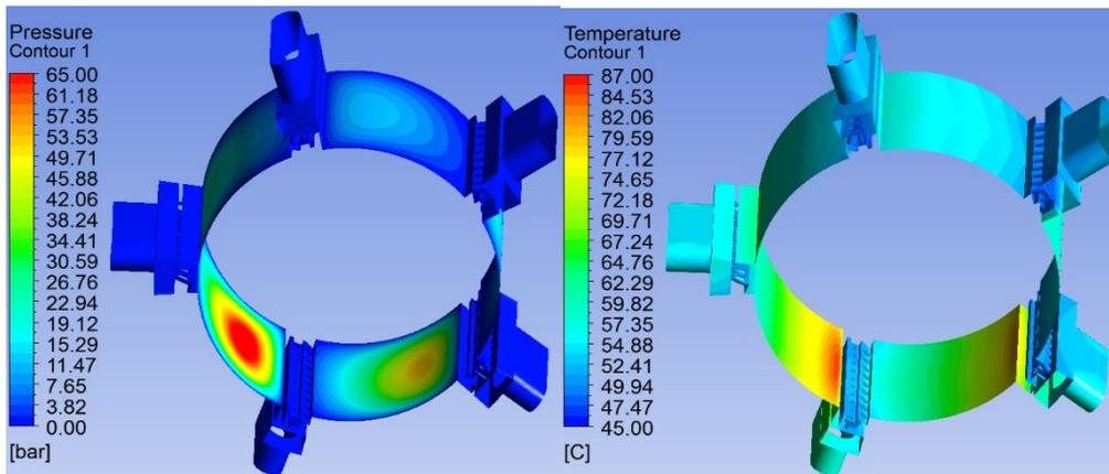
Fig 3 - Distribution of temperature and oil pressure in an oil supply pocket presented by CFX simulation
