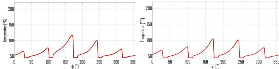
Fig 11 - Temperature of lubrication film pressure calculated by Miba with warm oil reduction of 30% and with 90%.
