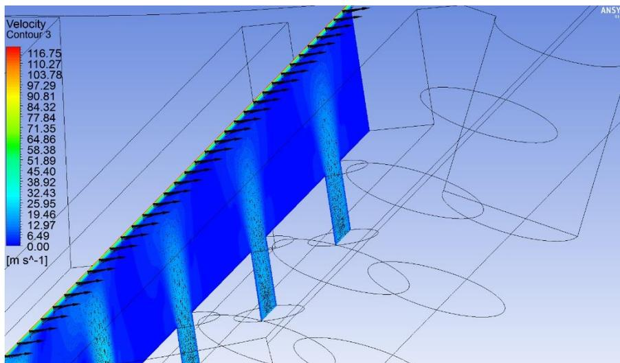
*Fig 9 – Local effectiveness of oil nozzles over the width of the pad.*
