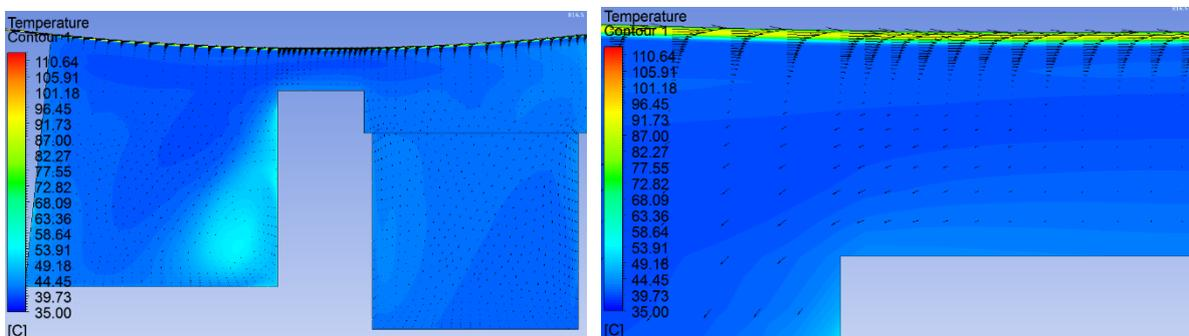
Fig 7 – Distribution of temperature and oil flux vectors in an oil supply unit according to design E1. Flow back of fresh oil between dam and shaft towards previous pad.
