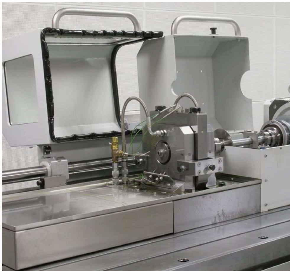
FIGURE 5 Engine bearing test rigs designed to overload bearings for functional tests such as misalignment (© Miba)
