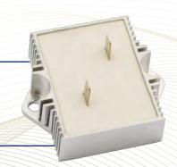
A PREcharge circuit allows the current to flow in a controlled manner until the voltage level rises to a value close to the source voltage before the main contactors close. This precharging normally takes place within one second by limiting the inrush current. To limit the inrush current, power resistors are used in combination with a relay. As soon as the capacitors have reached the operating voltage, the pre-charging relay opens and interrupts
