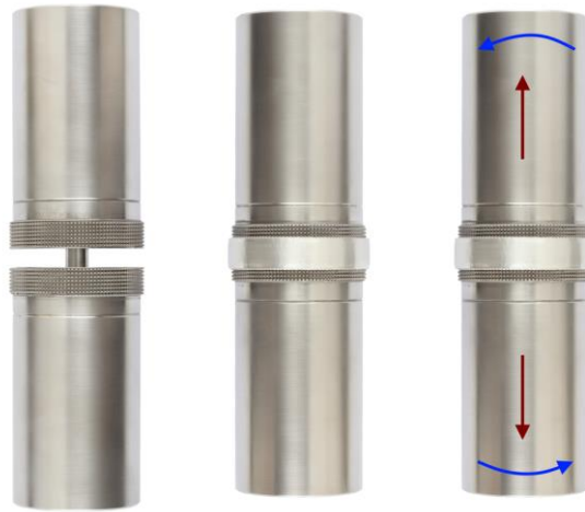
Figure 8: Split-shaft setup for mechanical characterization
