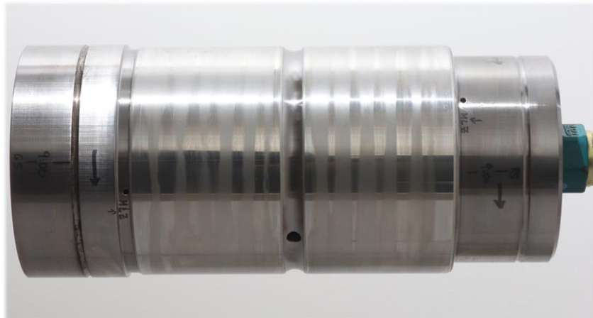
Figure 7: Crimped pin after GBX validation test
