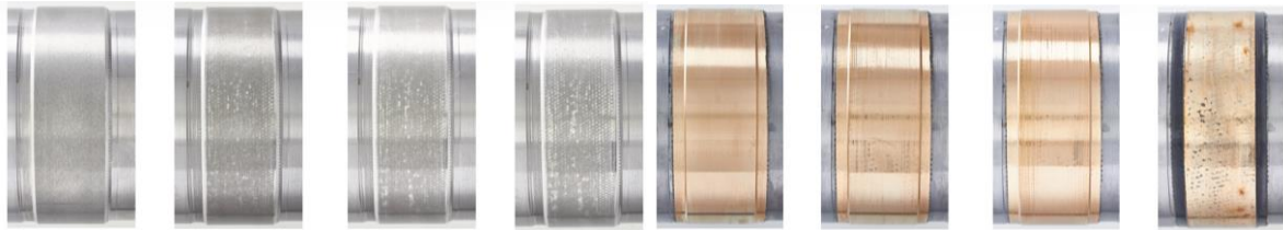
Figure 6: Optical appearance of AlSn20 (left) and CuSn12 (right) specimen after load limit identification at 0.5m/s in comparison with untested specimens.
