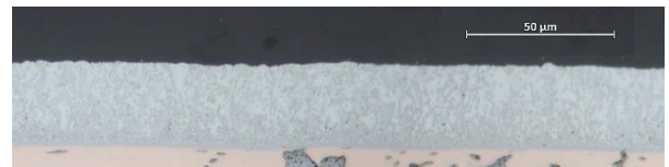
Figure 40. b) Detailed view of the sputter layer at the reference area
