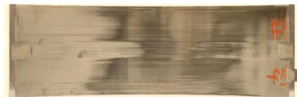
Figure 42. b) A Miba3B lower main bearing underwent 8330 MWh operation in the same locomotive as Figure 42a
