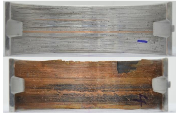
Figure 5. Numerous particles scorings (upper) and seizure (lower) of main bearing lower shells in a high-speed diesel engine
