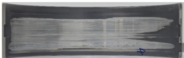
Figure 41. a) A lower main bearing (Miba61) underwent 100hours test in a high-speed propulsion engine
