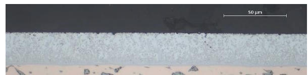
Figure 40. b) Detailed view of the sputter layer at the reference area
