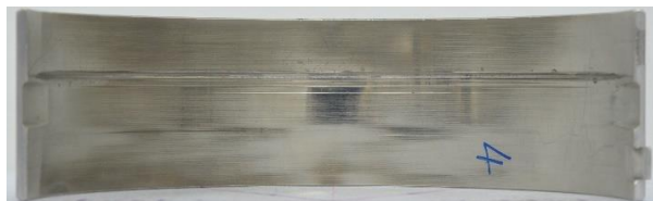
Figure 41. b) A lower main bearing (Miba3B) underwent 500hours test in a high-speed propulsion engine
