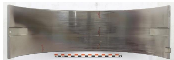
Figure 40. a) A lower main bearing (Miba3B) underwent 12000 hours test in a high-speed genset
