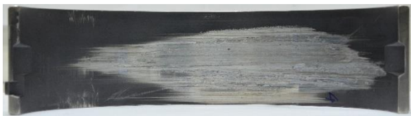
Figure 4. Mixed friction in the bearing center of a main bearing lower shell in a high-speed diesel engine
