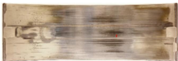
Figure 42. a) A Miba03 lower main bearing underwent 4389 MWh operation in a locomotive
