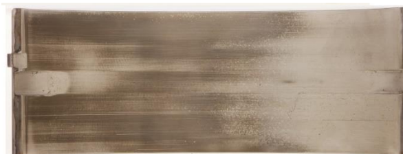
Figure 43. b) A Miba3B upper rod bearing underwent 7500 MWh operation in the same locomotive as Figure 43a
